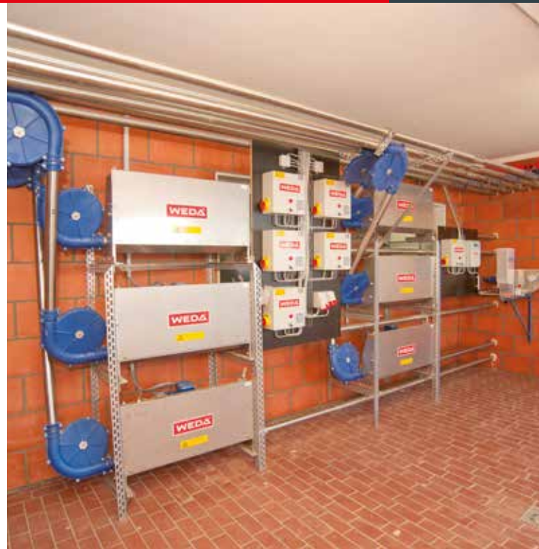
Control centre of dry feeding system with 6 feed lines
